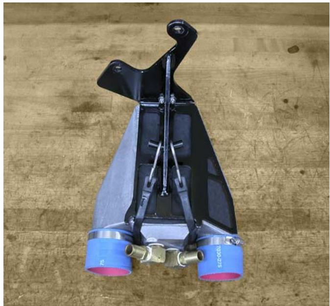
Apply silicone sealant to surface area of mounting bracket that will be placed against hull. Install and secure Power Cooler/Mounting Bracket assembly using stock hardware. **NOTE: Apply red Loctite to bolts. Torque to 61 N•m (45 ft•lb).**
