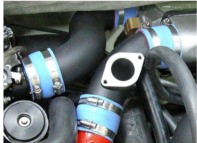
At this point you are left with installing your option for the mounting flange on the supercharger discharge tube. RIVA Racing strongly recommends the use of a Blow-off Valve to prevent unnecessary wear on the supercharger clutch. We offer the following options:
